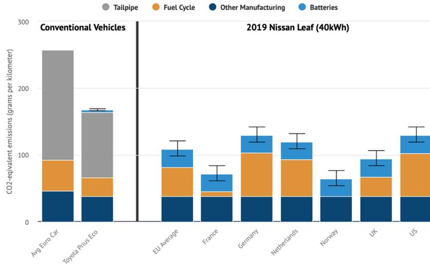
Lifecycle GHG emissions from the 40 kWh Leaf are 50% lower than a gas vehicle that averages 7,2 L / 100 km in USA
