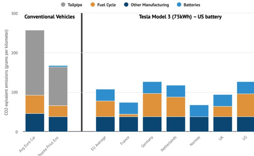
Lifecycle GHG emissions from a 75 kWh Tesla Model 3 are 43% lower than a gas vehicle that averages 7,2 L / 100 km in USA
