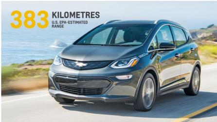
The Chevrolet Bolt EV set the range benchmark for an affordable EV capable of going the distance by delivering an U.S. EPA-rated 383 kilometres (238 miles) on a full charge.
